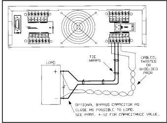
Figure 4-5. Remote Voltage Sensing
